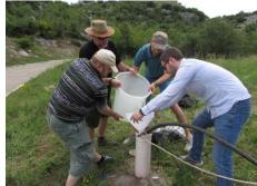
Preparation and injection of NaCl into the piezometer
