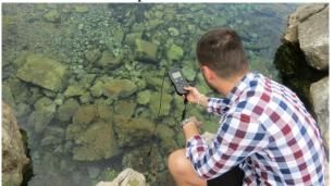
Monitoring of electrical conductivity on the spring
