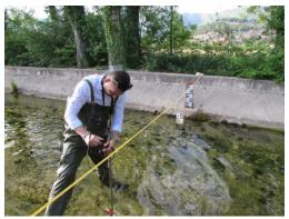
Measurement of spring discharge using current meter
